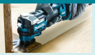
High operation efficiency thanks to large oscillation angle and constant speed control
